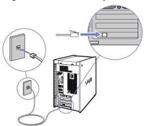
A country-specific phone plug is supplied with your VAIO desktop, allowing you to plug the phone line into the wall jack. We recommend you to use the supplied plug, because the usage of any other phone plug can decrease the connection quality.
